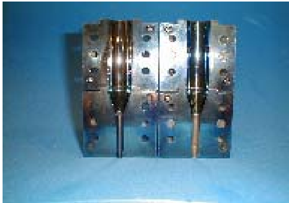
Figure 4. Die used in “The Carrot Scorch Test”.
