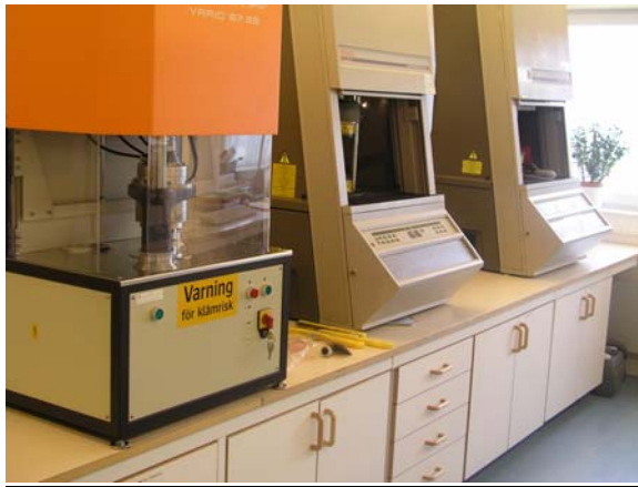
Fig. 8 Instruments to measure cure behaviour; Göttfert, Monsanto MDR and Monsanto ODR
