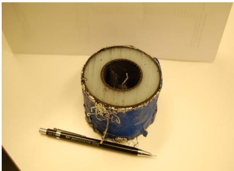
Figure 4: Picture highlighting XLPE cable insulation without the core.
