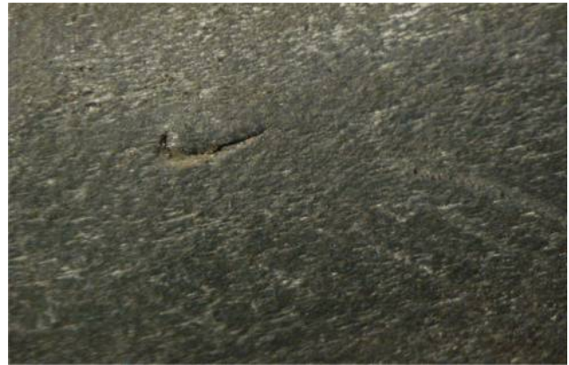
Figure 7 Cross-section image showing a transverse crack in the PVC jacket (40×)
