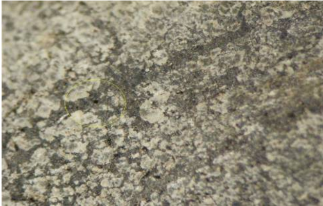
Figure 4 Cross-section of the outer PVC jacket showing air inclusions at the inner and outer surfaces (18×)
