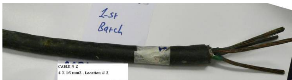
Figure 2 Typical example of a failed XLPE cable obtained from the site
